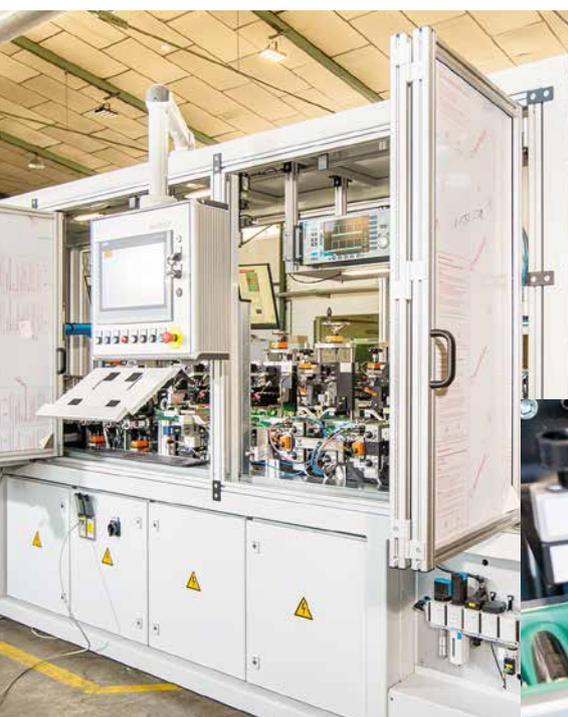
Robot controlled inspection system with ELOTEST PL600, ELO\SCAN and image processing module ELO\IMAGE.
