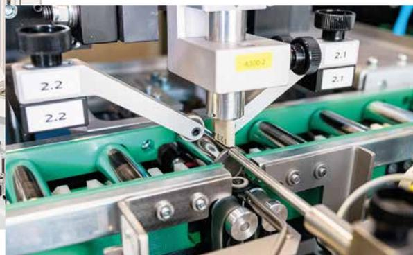
Automated inspection for cracks and grinding burns on rolling elements with the ELOTEST PL600 and probes (Type KD-129 and KDA-129).
