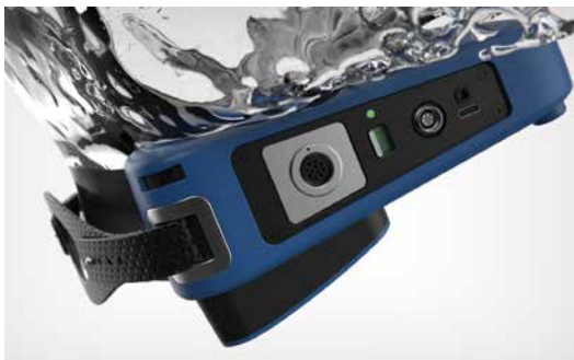
Protection class IP67 makes ELOTEST M6 best suited for offshore operation.
