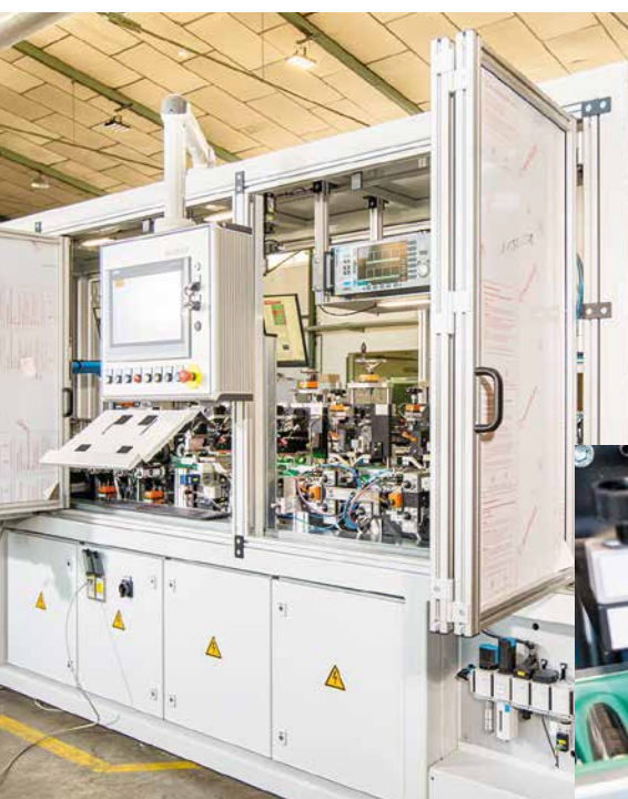
Robot controlled inspection system with ELOTEST PL650, ELO\SCAN and image processing module ELO\IMAGE.
