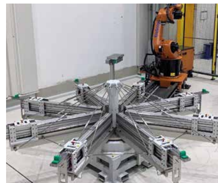
ELOSCAN application for components for the aerospace industry, Ø from 3.5 m up to 5.4 m.
