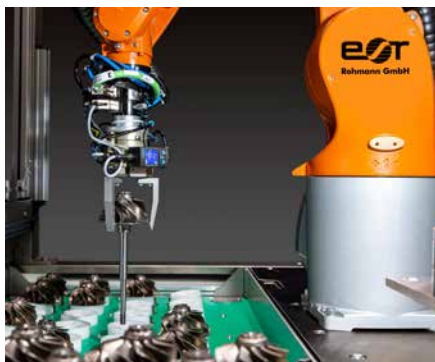
ELOSCAN Compact for the inspection of turbine wheels in the automotive industry.
